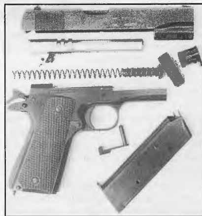
Norinco M1911A1 .45 ACP pistol, field-stripped.
